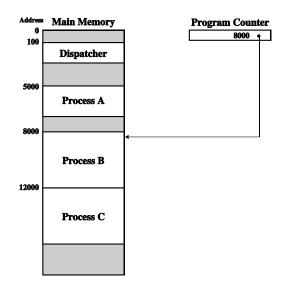
Figure 1: Main memory layout for multiprogramming
