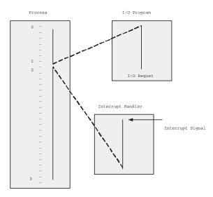
Figure 2: The typical dynamic behavior of a process
