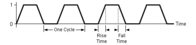
A **clock cycle** refers to a single complete traversal of the signal, from the rising edge, through the time when the value of the clock is one, through the falling edge, the time that the value is zero, until the start of the next rising edge. (You can actually "chop" the signal wherever you want and have it be a single cycle, as long as you only cover one cycle without "overlapping").
